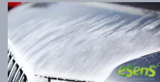
Foaming product recommended to break down ground-in dirt. Applied by a second nozzle circuit 3 bar [43.5114 PSI], 12,2 L/min [2.684 gpm].
