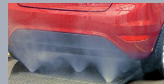
Two options are possible: static underchassis wash 10 bar [145.038 PSI], 90 L/min [19.8 gpm], and oscillating underchassis wash 15 bar [217.557 PSI], 120 L/min [26.4 gpm].
