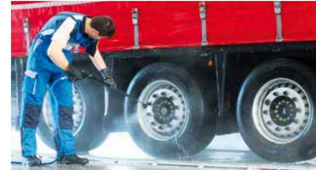
This optional extra allows the user to manually improve the automatic wash with a high-pressure gun working at **160bar** and with **18L/min**. Using the same gun, shampoo can be applied together with the high pressure, and a 15bar chemical prewash program can be selected. The external control panel can be mounted at a distance or wall-mounted. A reel can be installed too. The unit can work with hot water and with softened water.
