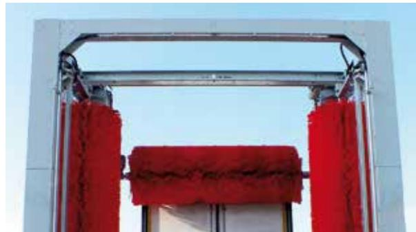
The optional high-density polyethylene horizontal brush completes the washing process on the front and the back of the vehicle, and it also washes the roof. It incorporates an anti-fall safety system, a frequency converter to control the elevation speed, and a transducer to control brush pressure, which ensures a perfect vehicle scan.
