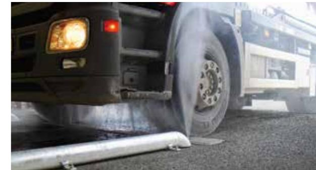
Drive-through underchassis wash with high-pressure system, 70bar and 126L/min. With entry photocells for an automatic operation and **12 rotating zero-angle nozzles**. Can be supplied from the same high-pressure pump rack as the lower side high pressure optional extra by means of a solenoid valve.
