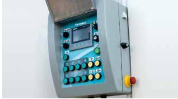
This optional external command post with a colour touch screen facilitates **navigation** on the machine menu. It consists of selector switches to turn on and off the vertical and horizontal brushes, push buttons to manually move the machine and the brushes, and program selection push buttons (up to 14 pre-set programs).
