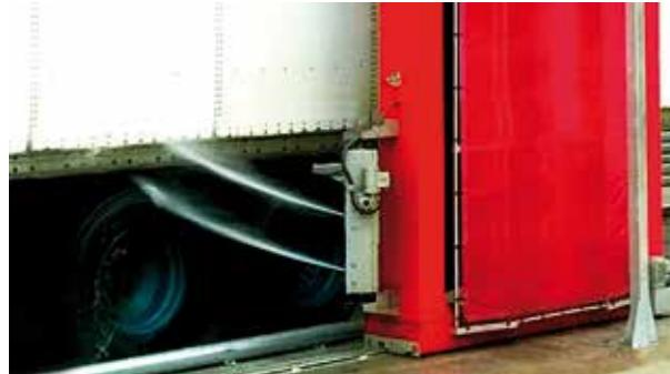
The perfect optional extra to complement the brush process in lower vehicle areas or on corners inaccessible to the brushes such as rims, underside, or tanks. It consists of **16 zero-angle nozzles** to operate at 70bar and with 84L/min. or 126L/min. It works with an oscillation motor (up-down) and a rotating cylinder (forward-backward) to thoroughly clean the area from different angles.
