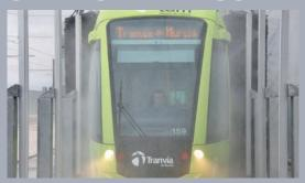
An optional extra designed to apply the chemical prewash product efficiently. Comprises two orientable pipes in stainless steel, nozzles with a non-drip system a dispensing system, and side protectors to minimise draughts and optimise the application of the chemical product.
