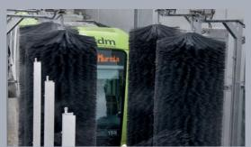
In addition to the group of four vertical brushes on the base module, 4 groups of 2 vertical brushes can be configured. These brushes are controlled by a programma-ble CPU, with electro-pneumatic pressure and spin force assistance sensors.
