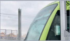
The perfect optional extra for the most complete of finishes. Its two orientable pipes spray the demineralised water all over the surface of the vehicles to remove any possible residue left over from the wash phase.
