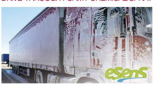
The optional drive-through foamy chemical sprayer includes the pipework and stainless steel protection screens. Hot application is recommended for greater chemical effectiveness with our specific **esens®** range for commercial vehicles. The unit includes a 100L [26,4 GAL] pre-mix tank and a high-pressure pump, 100 bar and 28L/min [1450 Psi and 7,4 GAL].
