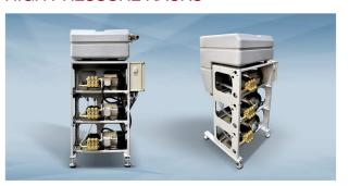
We have water pump racks for a high pressure wash at 70 bar [1015 Psi] and 126L/min [33,3 GAL], with 11 or 16.5kW [14,75 Hp or 22,12 Hp] total power, including -respectively- 2 or 3 70bar [1015 Psi] pumps with 5.5kW [7,37 Hp] power. They include a 200L [52,8 GAL] water tank at a high position to adequately supply the water pumps, and a by-pass valve with a pressure regulator. A 100 micron inlet filter protects the water pumps and prevents nozzles from clogging.
