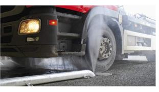
Drive-through underchassis wash with high-pressure, 70 bar [1015 Psi] and 126L/min [33,3 GAL]. With entry photocells for an automatic operation and 12 rotating zero-angle nozzles. Can be supplied from the same high-pressure rack used for lower side rotators provided the bay distance between the rotator module and the underchassis wash is adequate.
