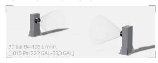
This version consists of 2 columns with electrically motorised high-pressure lower side rotators to ensure a constant spinning speed. The spraying arms include a stabiliser to avoid pressure losses during the wash process. With a working range from the ground from 250mm [10"] to 1.450mm [4'-9"], it is the ideal accessory to thoroughly clean the lower sides of vehicles used in transportation, civil works or mining.
