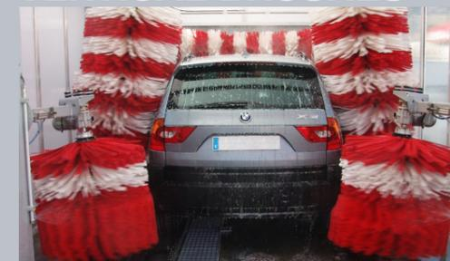
In installations from 12.5 meters, two additional vertical brushes can be installed to offer added value to the facility and higher wash quality. This option can be adapted to two different wash heights, 0.8 m and 1.6 m.
