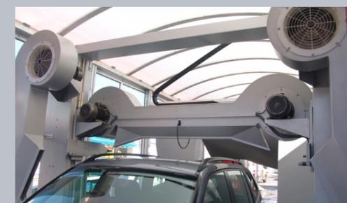
The dryer module is composed of 4 turbofans with 4 kW power each, working at low speed (1500 rpm) and with a high airflow rate for performance. The horizontal nozzle with its unique 3D design offers an exceptional dry quality with any type of vehicle.
